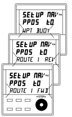
3. Use the **▼ STEP** knob select to the waypoint or the route to be used for navigation. The direction of the route is also selected by choosing ROUTE # FWD or ROUTE # REV (when NMEA data available via the Network PILOT, PILOT NMEA is also displayed).
