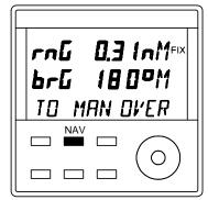
3. The display will now show the range and bearing to the MOB event. This display can also obtained by pressing the NAV key.
