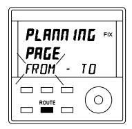
1. Press the **ROUTE** key until the display shows **PLANNING PAGE**, **FROM** and **TO** will be showing on the text display. **FROM** will flash.
