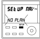
2. Press the **SETUP** key, the display will flash either **NO PLAN**, or one of the displays shown in 3.
