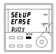
2. Press the **SETUP** key six times, the display shows **ERASE**.
