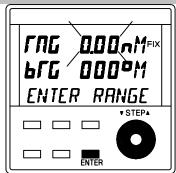
**3.** Press the **ENTER** key. The range in nautical miles will flash. Use the **▼STEP** knob to enter the range from 0.01 to 9.99nM.
