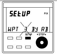
2. Press the **SETUP** key 5 times. The display will show **WPT### BY RB**. Use the ▼ **STEP** ▲ knob to select a **WPT** number.
