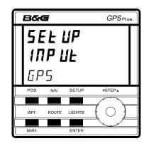
Press the **ENTER** key, the display will now show **nOt USEd**. Turn the **▼ STEP ▲** knob. If the GPS has not yet locked onto the position then **nOt USEd** will remain. If the GPS has locked then **nOt USEd** will be replaced with the Latitude and Longitude.
