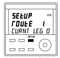
2. Press the **SETUP** key three times. The display will show the current leg number of the selected route, e.g. **CURNT LEG 0**.
