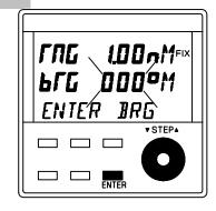
**4.** Press the **ENTER** key. The bearing in degrees will flash. Use the **▼ STEP ▲** knob to enter the bearing from 000° to 359°.
