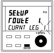
3. Press the **ENTER** key, the leg number will flash. Use the **▼ STEP** ▲ knob to select a different leg number.
