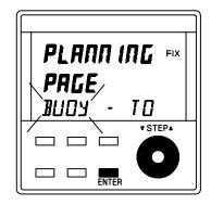
2. Turn the ▼ STEP ▲ knob to cycle through the waypoints in the library until the desired waypoint is displayed e.g. *BUOY*. Press the ENTER key to select the displayed waypoint. *TO* will now flash.
