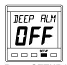
Press **SETUP** key, the alarm state will be displayed.
