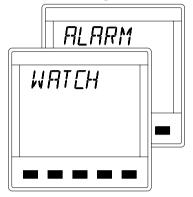
The Off Course alarm is activated when the boat deviates off course by a preset amount. The display alternates between the messages below:
