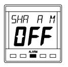
Press **ALARM** key to display shallow alarm **SHA A M**.
