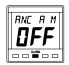
Press **ALARM** key to display anchor alarm **ANC A M**.
