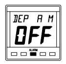
Press **ALARM** key to display shallow alarm **DEP A M**
