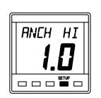
Press **SETUP** key 3 times to display **ANCH HI** value.
