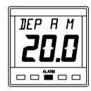
Press **ALARM** key, the alarm is displayed.
