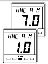
Press **ALARM** key to display the anchor alarm.
