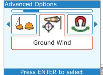
2. Press ENTER, to display the **Ground Wind** setup box.
