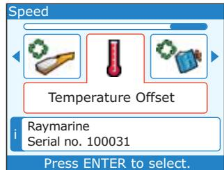
4. Press ENTER to display the **Temperature Offset** setup page.
