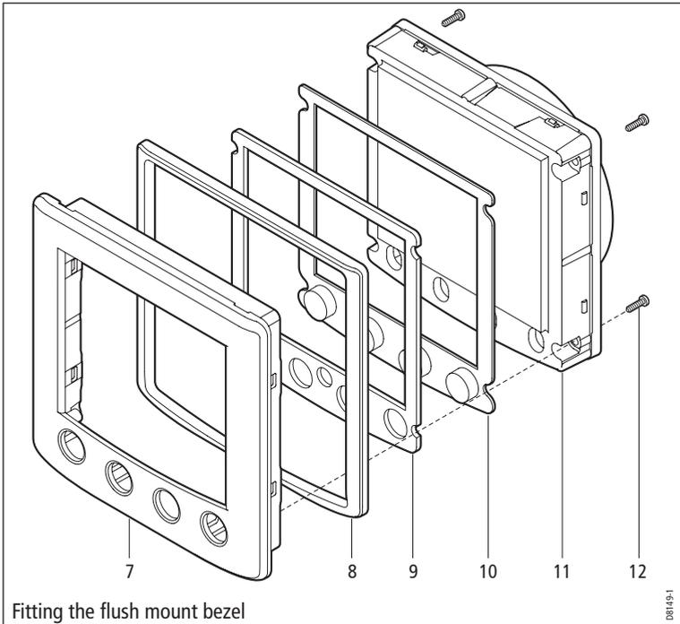
6. Place the assembled flush mount bezel and panel seal, in position on the instrument, so that the rubber keys are correctly located in the holes on the bezel, then clip the bezel and instrument together.
