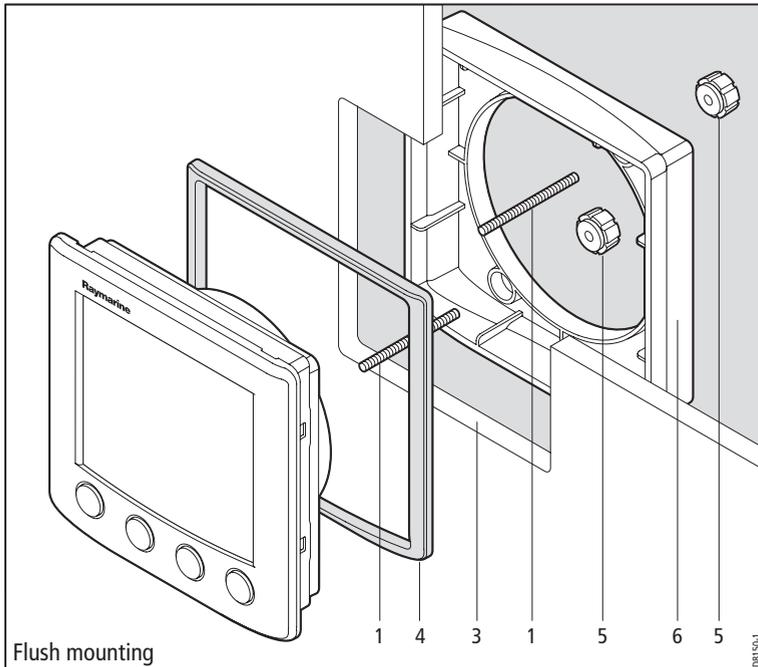
6. Screw the two fixing studs (1) into the threaded sockets on the rear of the instrument.
