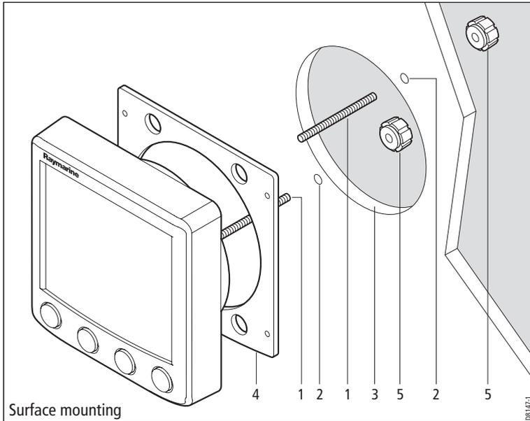
6. Screw the two fixing studs into the threaded sockets on the rear of the instrument.
