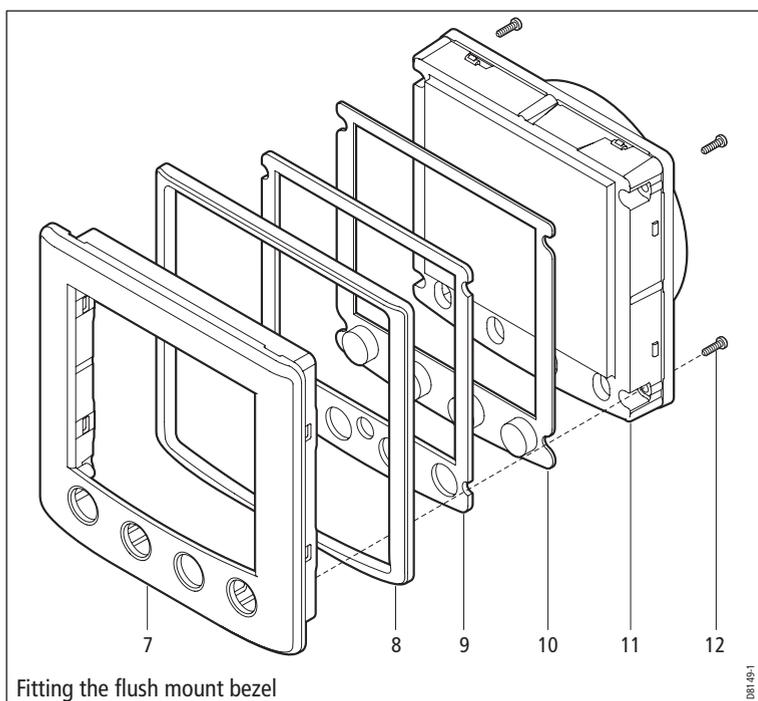
Fitting the flush mount bezel
