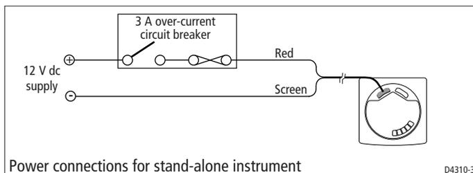
2. Run the power cable from the instrument to a suitable 12 V dc power source.
