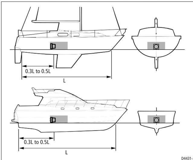
The Fluxgate Compass transducer must also be sited:
