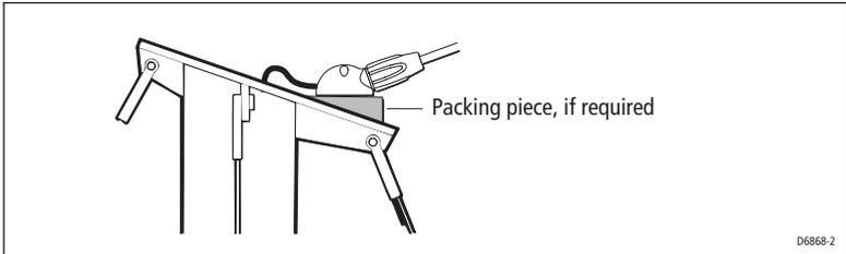
You can fit your wind vane so the cable leaves the wind vane base either from the rear (option A), or from underneath (option B), as in the following *Wind vane cable options* illustration.
