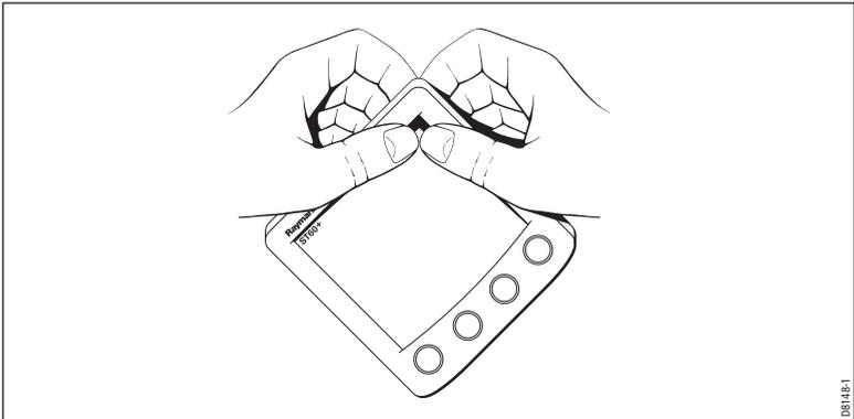
2. Using both thumbs, gently press an upper corner of the instrument from the bezel, then remove the bezel from the instrument. Retain the rubber keypad which is released when the bezel is removed.
