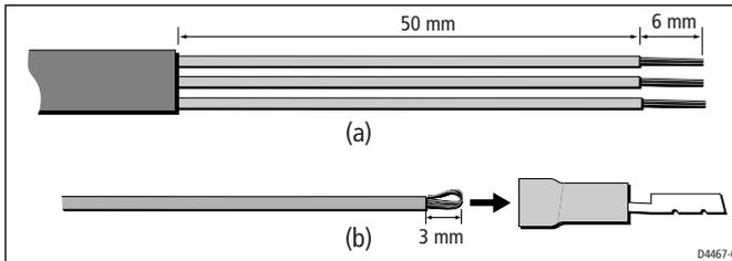
Referring to the *Connections to ST60+ Club House Wind instrument* illustration, connect the Wind Vane cable to the instrument.
