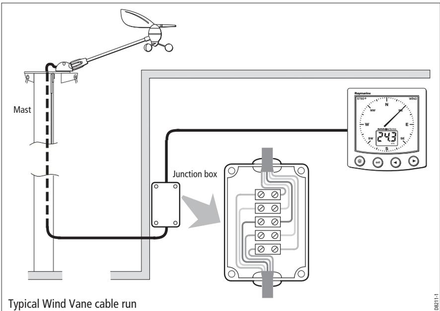
The Wind Vane is supplied with sufficient cable already connected, to run from the mounted position to the ST60+ Club House Wind instrument. The manner in which you run the cable will depend on the locations of the transducer and instrument. The following guidelines are provided:
