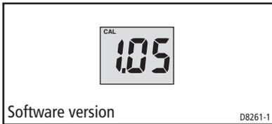
2. Note the software version number, then hold down the **⌘** and **set** buttons for approximately 2 seconds, to return to normal operation.
