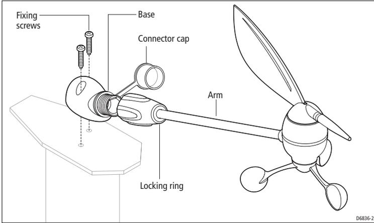
3. Referring to the *Wind vane cable options* illustration, route the cable correctly for the option you are using, then secure the wind vane base, using the two self-tapping fixing screws.
