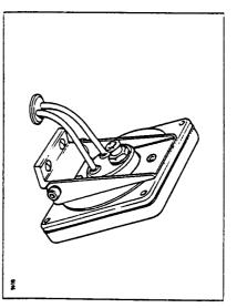
position protected from the weather. When bracket mounting the instrument it must be mounted in a sheltered
