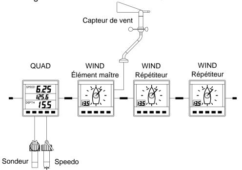
Network SPEED, Network DEPTH, Network WIND and Network TACK (magnified wind angle).
