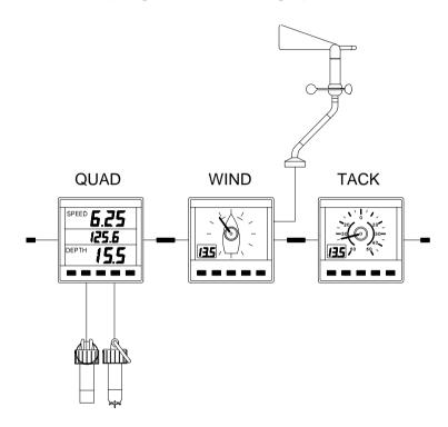
The Network units can be connected together in any order as data is shared via the system network cable link.
