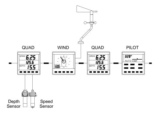
If the Network QUAD unit losses valid depth data, due either the actual depth being outside the working range, or to extreme turbulence in the water the LCD will show 3 "floating" bars. This shows that the unit is attempting to calculate the depth and is still functioning.
