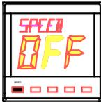
If there is no speed data the Network DATA unit will display **OFF** when the **SPEED** key is pressed.
