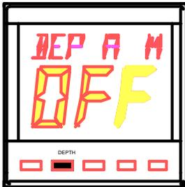
The Network DATA unit can display the alarm value that has been set or **OFF** if it is not enabled. The following are examples of a depth alarm displays. See USING THE DEPTH KEY for all the available alarm displays.
