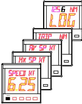
Press the **SPEED** key to cycle through the speed options.
