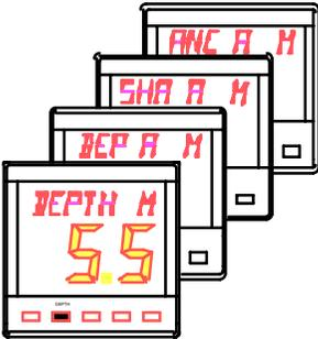
Press the **DEPTH** key to cycle through the depth options.
