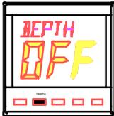
If there is no depth data the Network DATA unit will display **OFF** when the **DEPTH** key is pressed.
