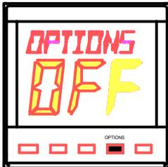
If there is no data available the Network DATA unit will display **OFF** when the **OPTIONS** key is pressed.
